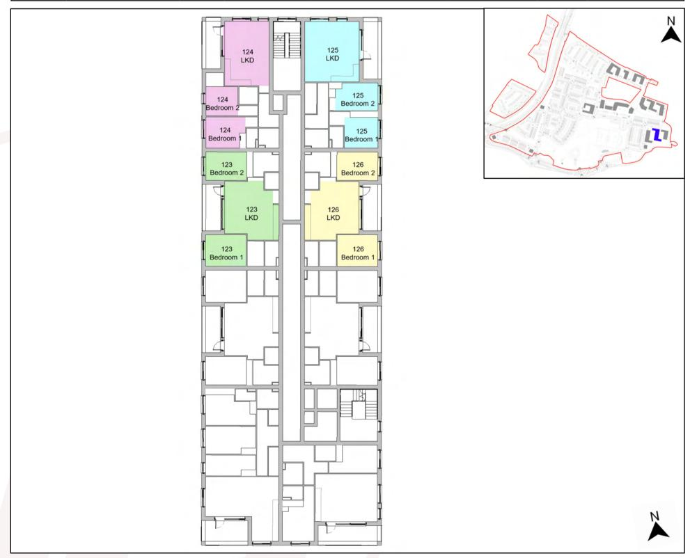
Figure 7.95: Floor plan of assessed building & Keyplan highlighting the assessed building.
