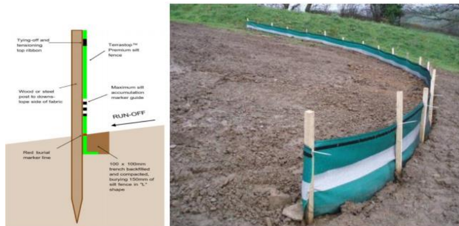
Figure 13: Silt Fence
