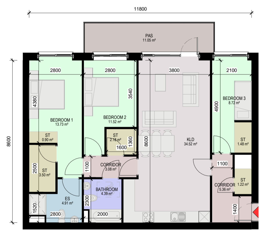
8 APT A3/5- 11-Floor Plan - 3 BED, 5 PERSON APARTMENT - NET INTERNAL AREA (NIA) - GROSS INTERNAL AREA (GIA) - 101.3m² 1: 100
