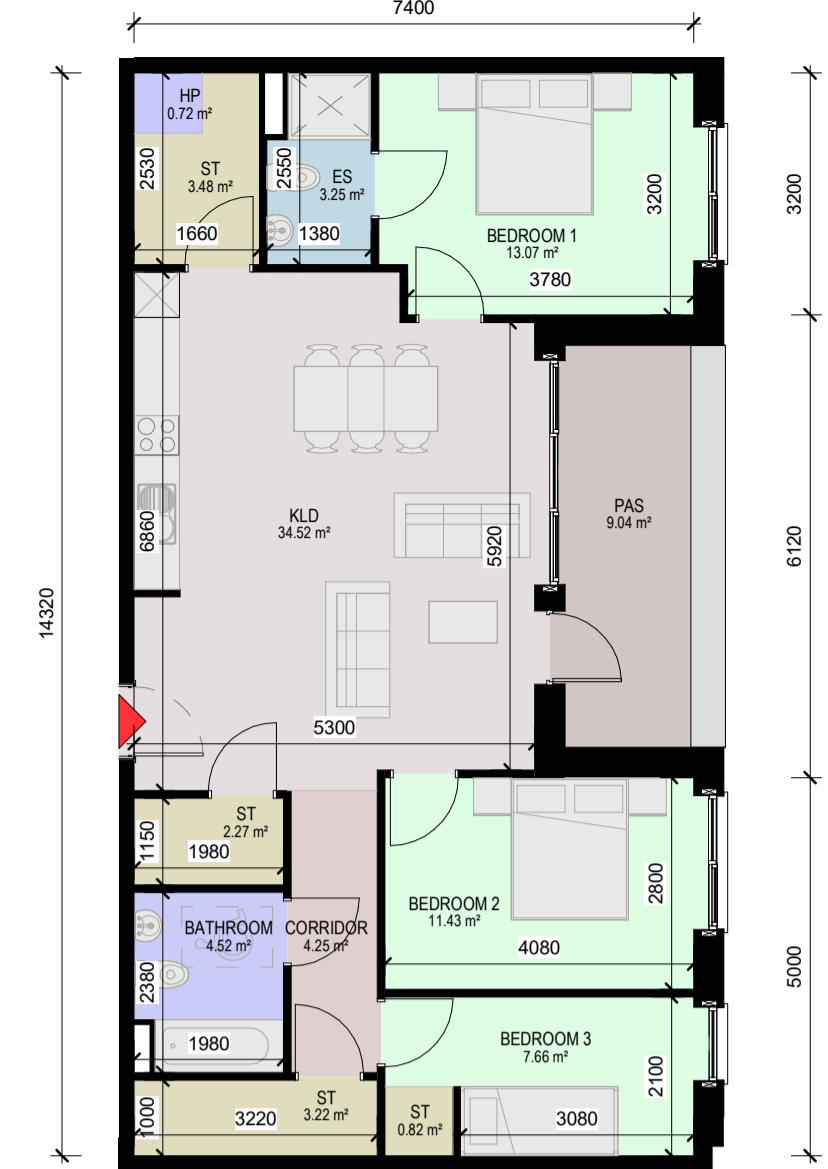
3 APT A3/5- 15-Floor Plan - 3 BED, 5 PERSON APARTMENT - NET INTERNAL AREA (NIA) - GROSS INTERNAL AREA (GIA) - 93.1m² 1: 100
