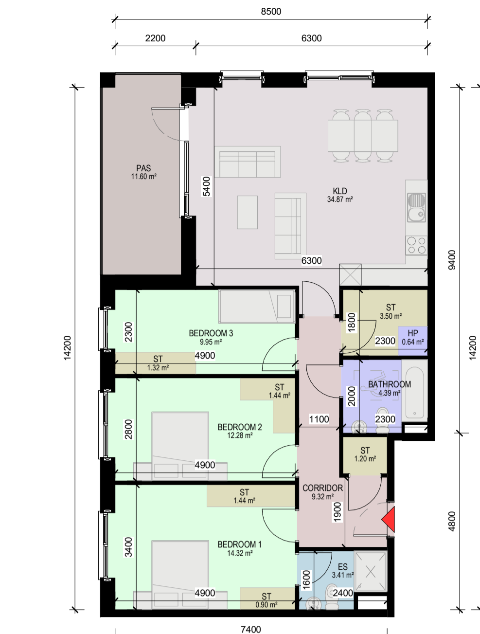
1 APT A3/5- 1-Floor Plan - 3 BED, 5 PERSON APARTMENT - NET INTERNAL AREA (NIA) - GROSS INTERNAL AREA (GIA) - 103.3m² 1: 100
