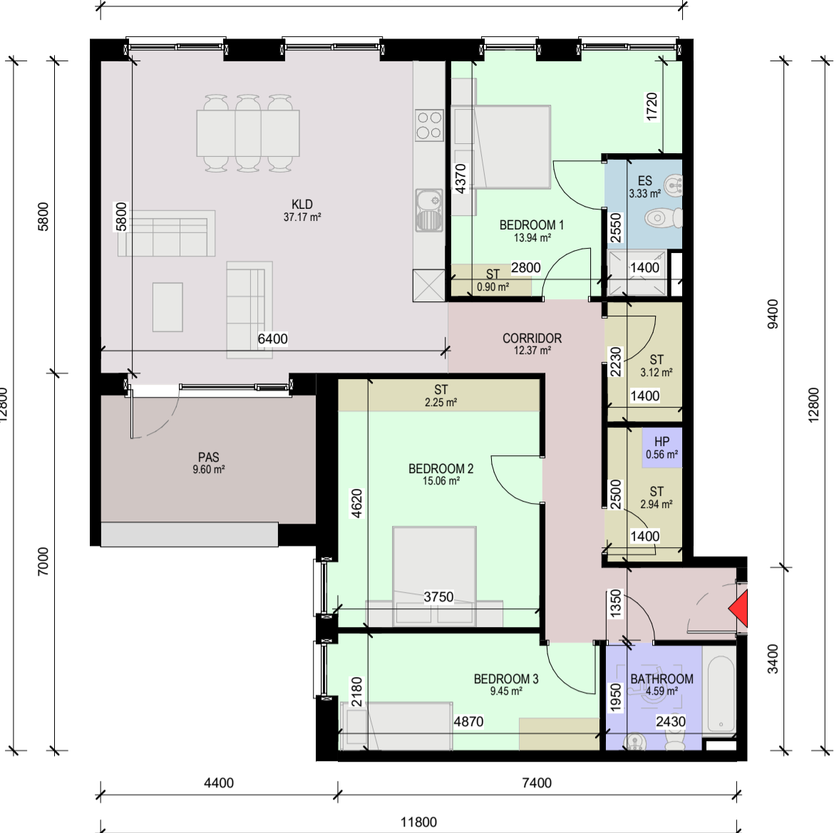
4 APT A3/5- 21-Floor Plan - 3 BED, 5 PERSON APARTMENT - NET INTERNAL AREA (NIA) - GROSS INTERNAL AREA (GIA) - 110.8m² 1: 100
