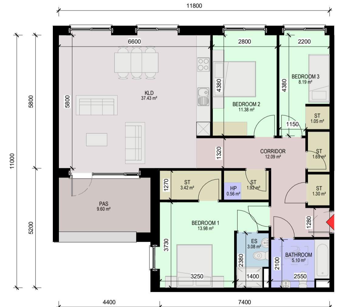
7 APT A3/5- 24-Floor Plan - 3 BED, 5 PERSON APARTMENT - NET INTERNAL AREA (NIA) - GROSS INTERNAL AREA (GIA) - 106.9m² 1: 100
